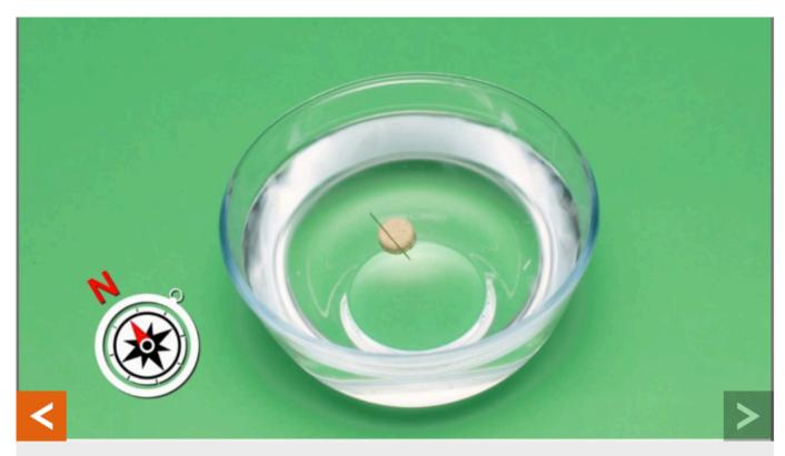
The needle will turn and then come to a complete stop. It will be facing magnetic north. You can check this by placing the compass next to the bowl.
